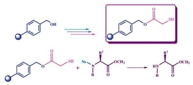
A solid-supported thiol has been conveniently prepared by treating an S-protected mercaptoacetic acid with Wang resin. Deprotection of the thiol function pro-
